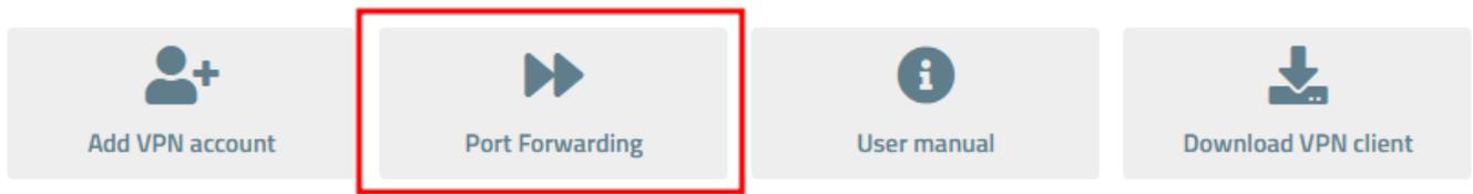
To create a new port forwarding rule, enter the port you want to forward, select the protocol, choose the VPN account from the dropdown list to which the port will be forwarded, and enter the port to which the forwarding will occur. After filling in the details, press the "**Add Port Forwarding**" button.
